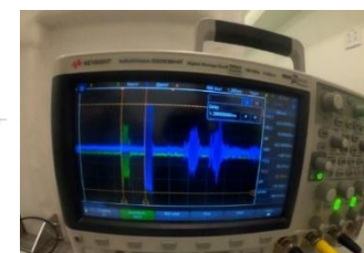
Time of Flight Delay Verification
